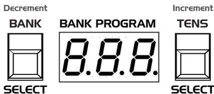
Use the Bank/Decrement and Tens/Increment buttons to scroll forward and backward, respectively, through parameter settings
