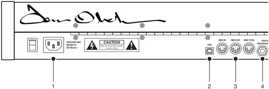
**1. AC Power Connector**—Accepts a standard, grounded IEC power cord. Operates over a range of 100 to 240 volts and 50 to 60 Hz.
