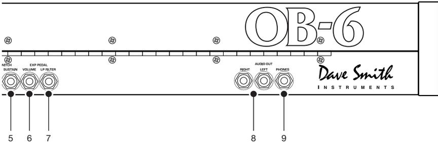
**6. Expression Pedal-Volume**—Accepts a standard expression pedal that has a variable resistor on a TRS (tip-ring-sleeve) ¼ inch phone plug. Once connected, you can use the pedal to control volume to add expressiveness and dynamics to live performance.
