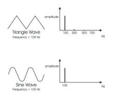
Like the square wave, the triangle wave only contains odd harmonics, but the levels of the harmonics in a triangle wave are much less. The triangle wave has a soft, slightly buzzy sound that is suitable for highpitched leads (like a flute) or adding a beefy sub-bass to bass sounds.
