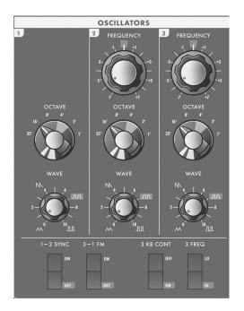
Oscillator I performs as a master oscillator to which Oscillator 2 and 3 are tuned. The timbres of the oscillators are adjusted by their variable Waveform controls. In addition, there are switches for Oscillator 2 sync to Oscillator 1; linear frequency modulation of Oscillator I by Oscillator 3; Oscillator 3 keyboard control ON/OFF; and Oscillator 3 Lo or Hi frequency range.
