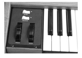
The Voyager OS has a 44-note keyboard ( $3\frac{1}{2}$  octaves, F to C), just like the original Minimoog. The Voyager's keyboard produces velocity and aftertouch (pressure) voltages monophonically. These voltages can be used as modulation control signals through the Modulation Busses, or as external control signals when the Voyager is connected to the optional VX-351 CV Expander.
