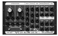
The VX-351 Voyager CV Expander is an add-on product that expands your Voyager OS into a semi-modular synth. The VX-351 contains all of the Voyagers CV and Gate *outputs* on 1/4" jacks (19 CV outputs and 2 Gate outputs). In addition, there are two active attenuators for reducing or inverting the strength of a CV signal, and two 4-way Multiples for sending a single CV signal to multiple control destinations.
