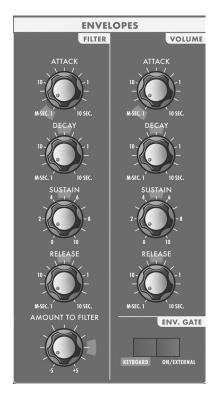
When triggered, EG's produce a time-varying control voltage that has a specific start, middle and end profile. The four parameters that define this profile are Attack, Decay, Sustain and Release, sometimes abbreviated as ADSR.
