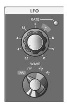
For the Sample and Hold circuit, the LFO's square wave is used as the S&H Trigger input, while the Voyager's Noise source is used for the S&H Input signal. For each positive-going cycle of the LFO square wave, the voltage at the input of the S&H circuit is sampled and held until the next cycle. Since the sample source is Noise (a random signal), the voltage that appears at the output of the S&H circuit is a random voltage that changes in time with the LFO.
