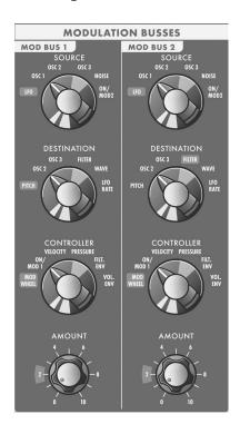
The Modulation Busses allow you to select a variety of modulation sources, destinations, modulation controllers, and amounts. The two Mod Busses are labeled MOD BUS I and MOD BUS 2, and are identical in function. The control of each mod buss is selectable instead of being tied to a particular controller, and six controller options are available.
