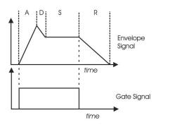
The second auxiliary component is the Envelope Generator, or EG. The EG makes no sound by itself. Rather, it creates a time-varying control voltage that is typically used to control the gain of the amplifier, or the cutoff frequency of the filter. Many synthesizers, including the Voyager, provide several EG's for independent envelope control of the amplifier and filter circuits.
