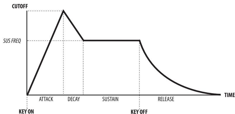
**Attack:** determines the time to reach the maximum filter cut off frequency, that is also determined by other parameters (ref: amount).
