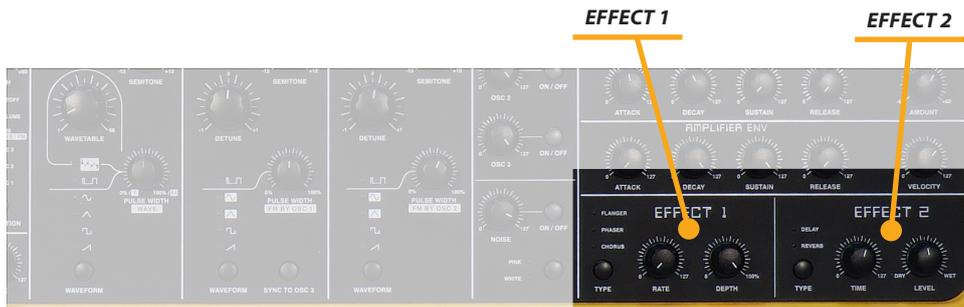
**Chorus:** this warm and rich effect is generated by using Comb filters that creates slightly detuned copies of the input signal and mix it into the output signal. The result sounds like an ensemble of several simultaneous sounds, like a choir as opposed to a single voice; hence the name Chorus. The detuning is generated by an internal LFO that can be controlled in Rate and Depth by the related potentiometers of the front panel.
