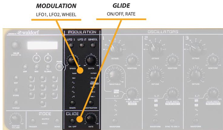
**Shape:** by using the Shape button, the user can select the related shape of the Modulating waveform, from the Sawtooth to the Random generator; please note the a sine wave or a triangle is generally used for obtaining symmetrical effects (such as Vibrato or Tremolo) while the other shapes are selected by the user's taste or sound research targets. The Speed and Depth controls do effect the related parameters.
